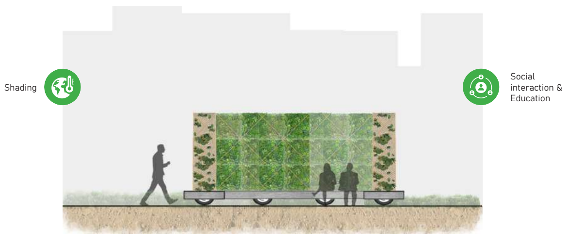
Fig 4.15 Detail of a typical mobile vertical greening unit and its associated benefits.
