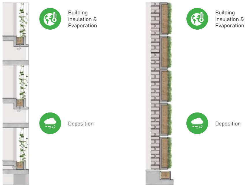
Fig 4.10 Two types of façade-bound greening. Planter-based with climbers (left) and a modular greening system (right).
