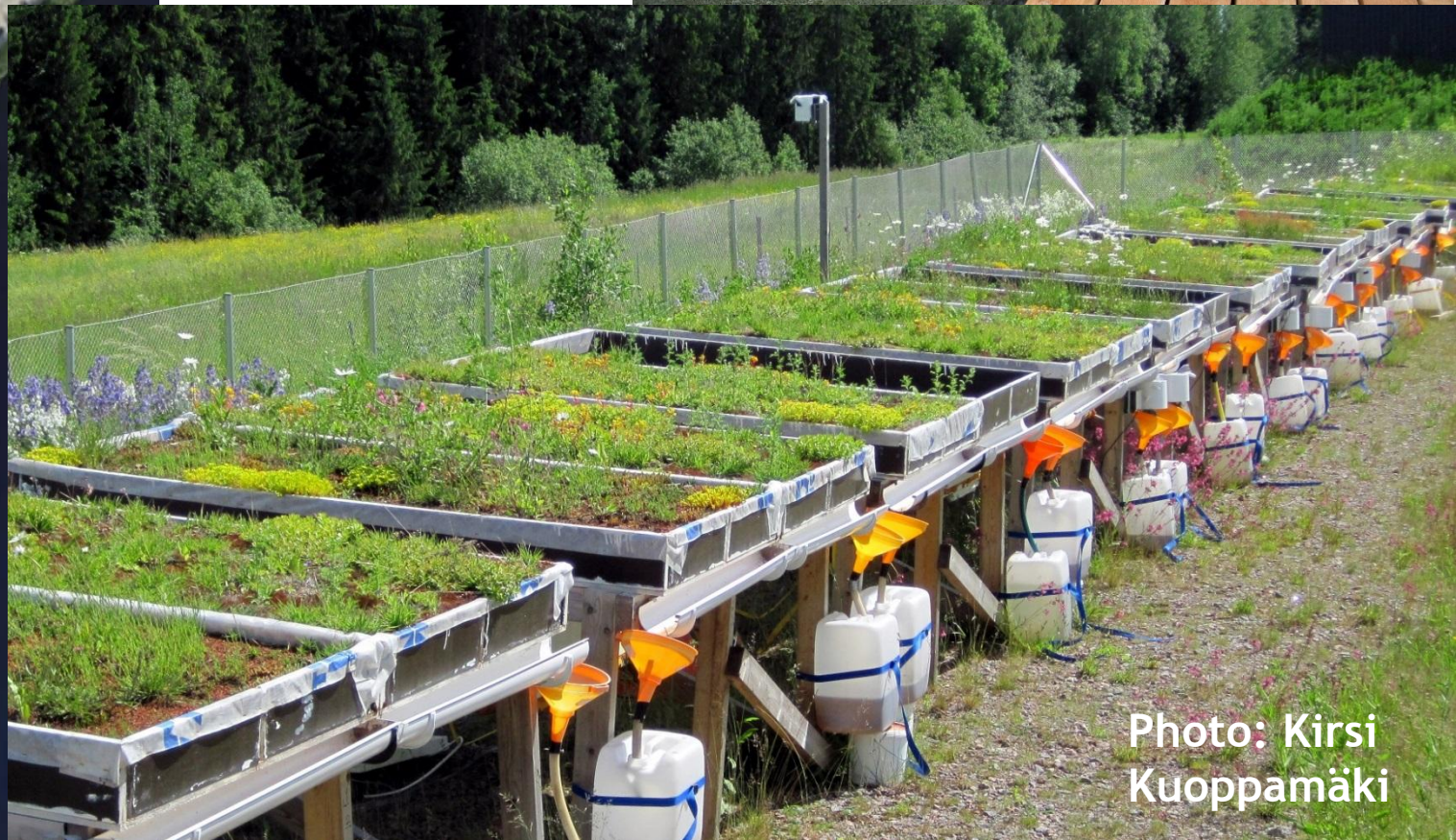
Biofilter demo 2018 for leakage waters from contaminated site
