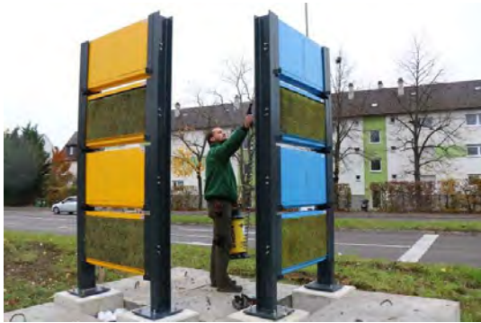
MoosTex: Test site for pollution absorbing noise protection wall 30
