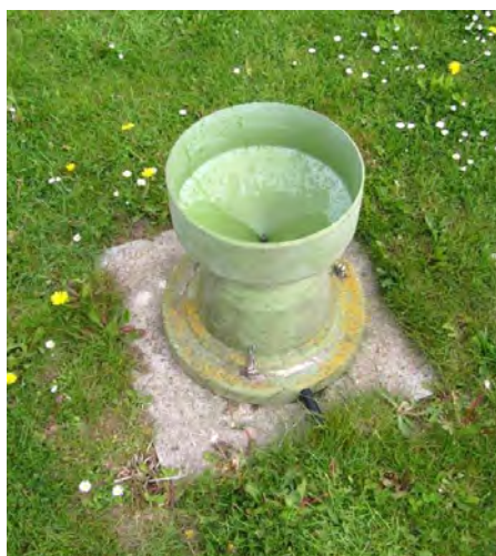
Figure 11. Tipping-bucket rain-gauge (reproduced from Met Office, 2010)
