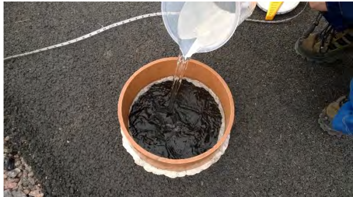
Figure 13. Left: Dimensions of the infiltration ring per ASTM C1701/C1701M-09 standard test method. Right: Infiltration rate measurements on a permeable asphalt conducted by VTT Technical Research Centre of Finland Ltd
