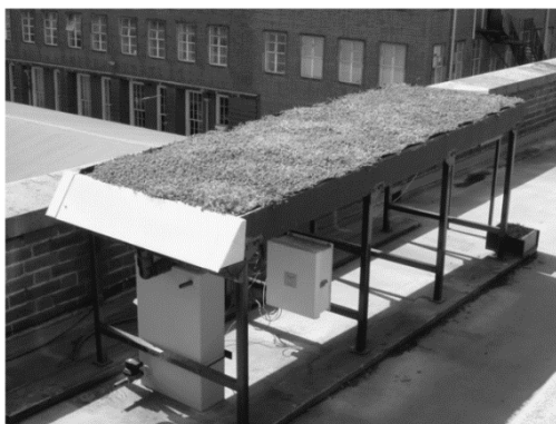
Figure 6. Green roof performance monitoring test bed (reproduced from Stovin et al., 2012)
