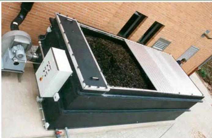
Fig. 105: Biofilter (source: FUCHS Enprotec GmbH; www.fuchs-germany.com)
