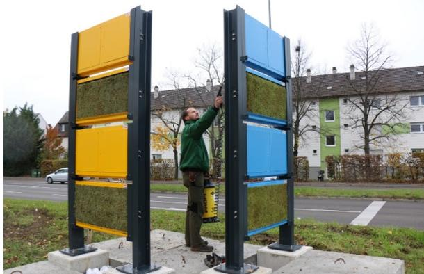
Fig. 32: MoosTex: Test site for pollution absorbing noise protection wall (source: Helix-Pflanzen)
