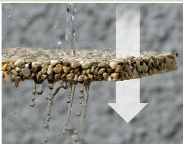
Fig. 65: Permeable stone carpet (source: [www.drenatech.it/](http://www.drenatech.it/))
